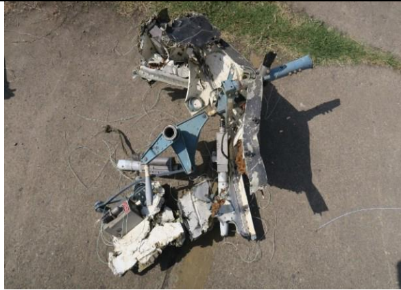
L/H cyclic pitch stick and L/H roll channel bellcranks
