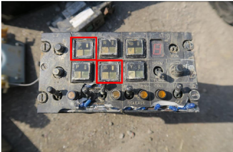
AUTOPILOT CONTROL PANEL
