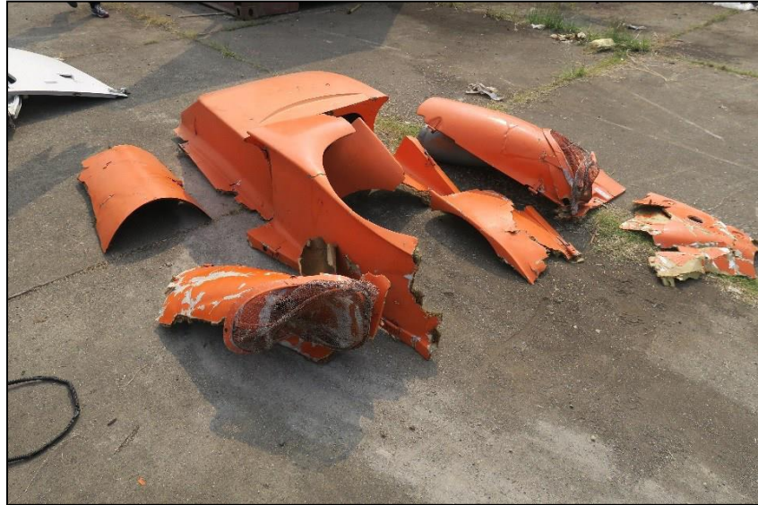
Damage to the front and right side part of the MGB cowling
